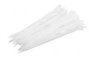
Cable ties are made with type 6/6 nylon for high impact and tensile strength. They are self extinguishing -UL 94 Flam. Class V2 and non-corrosive. Operating temperature from -40°F to 185°F (-40°C to 80°C). Heat stabilized from -40°F to 221°F (-40° to 105°C)
